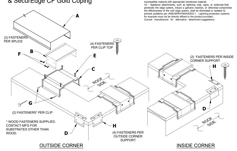
NOTE: ALL MITERS, END CONDITIONS, AND ACCESSORY CONDITIONS SHOULD BE INSTALLED PRIOR TO STRAIGHT SECTIONS
