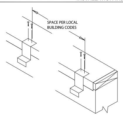
LOCATE AND FASTEN LIGHTNING ROD BRACKETS TO INSIDE FACE OF WALL PER LOCAL BUILDING CODES WITH APPROPRIATE FASTENERS FOR SUBSTRATE.
