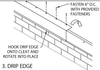
HOOK DRIP EDGE OF EACH DRIP EDGE SECTION ONTO CONTINUOUS CLEAT, ROTATE INTO PLACE. FASTEN THRU PRE-SLOTTED HOLES 6" WITH PROVIDED FASTENERS.
