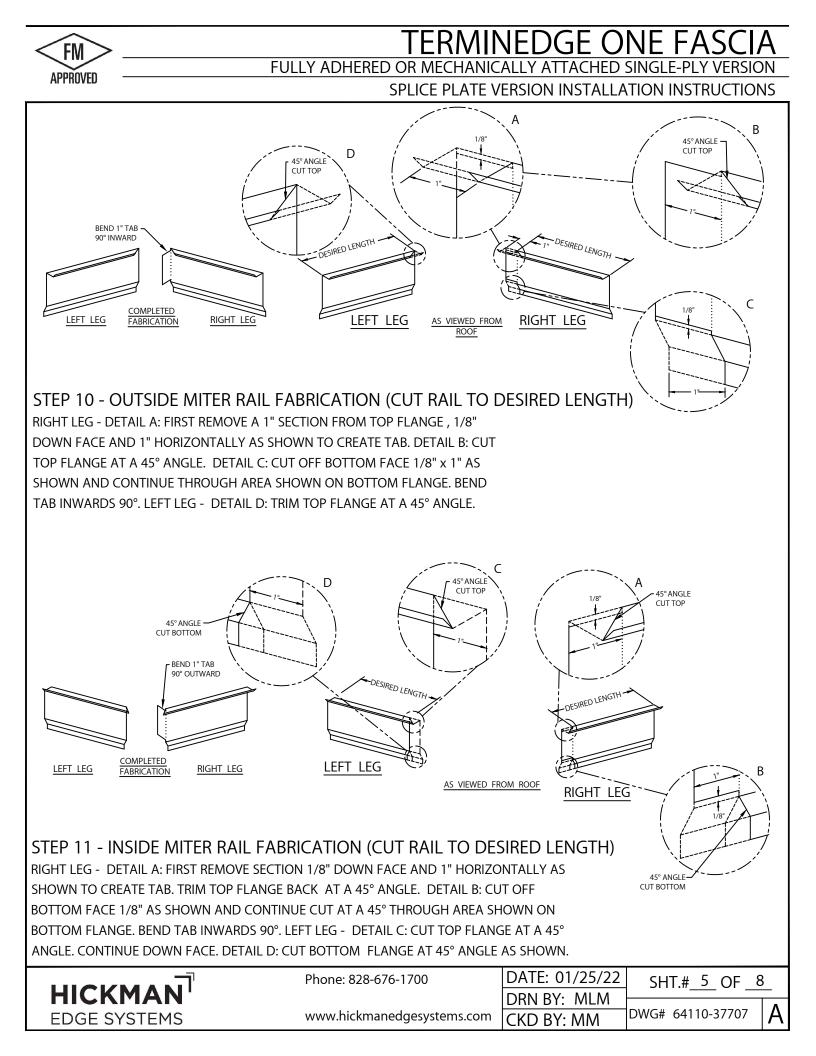
**TERMINEDGE ONE FASCIA** FULLY ADHERED OR MECHANICALLY ATTACHED SINGLE-PLY VERSION
