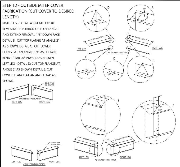
STEP 13 - INSIDE MITER COVER FABRICATION (CUT COVER TO DESIRED LENGTH)
