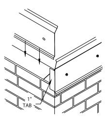
STEP 3 - RAIL MITER PREPARATION SEE PAGE 5 FOR MITER PREPARATION. FASTEN MITER BASE RAIL TO NAILER(S) THROUGH BASE RAIL SLOTS WITH PROVIDED FASTENERS.
