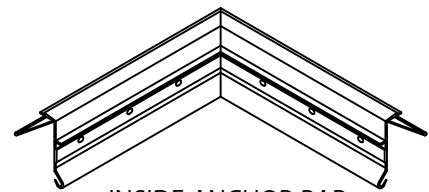
INSIDE ANCHOR BAR MITER
