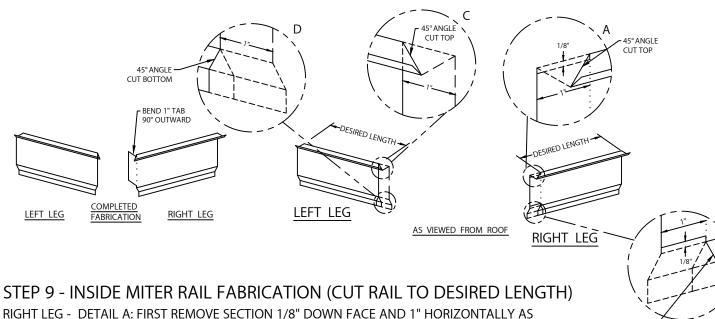
SHOWN TO CREATE TAB. TRIM TOP FLANGE BACK AT A 45° ANGLE. DETAIL B: CUT OFF BOTTOM FACE 1/8" AS SHOWN AND CONTINUE CUT AT A 45° THROUGH AREA SHOWN ON BOTTOM FLANGE. BEND TAB INWARDS 90°. LEFT LEG - DETAIL C: CUT TOP FLANGE AT A 45° ANGLE. CONTINUE DOWN FACE. DETAIL D: CUT BOTTOM FLANGE AT 45° ANGLE AS SHOWN.
