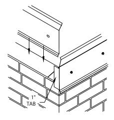
STEP 3 - RAIL MITER PREPARATION SEE PAGE 5 FOR MITER PREPARATION. FASTEN MITER BASE RAIL TO NAILER(S) THROUGH BASE RAIL SLOTS WITH PROVIDED FASTENERS.
