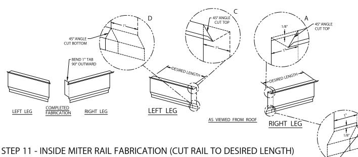
RIGHT LEG - DETAIL A: FIRST REMOVE SECTION 1/8" DOWN FACE AND 1" HORIZONTALLY AS SHOWN TO CREATE TAB. TRIM TOP FLANGE BACK AT A 45° ANGLE. DETAIL B: CUT OFF BOTTOM FACE 1/8" AS SHOWN AND CONTINUE CUT AT A 45° THROUGH AREA SHOWN ON BOTTOM FLANGE, BEND TAB INWARDS 90°, LEFT LEG - DETAIL C: CUT TOP FLANGE AT A 45° ANGLE. CONTINUE DOWN FACE. DETAIL D: CUT BOTTOM FLANGE AT 45° ANGLE AS SHOWN.
