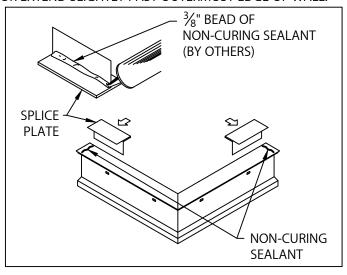
3. ANCHOR BAR MITER SPLICE PLATES APPLY A  $\frac{3}{8}$ " BEAD OF NON-CURING SEALANT (BY OTHERS) TO THE RIGHT ANGLE INTERSECTION OF THE DECK FLANGE AND TO EACH END OF ANCHOR BAR MITER. SLIDE 3½" WIDE SPLICE PLATE HALFWAY ONTO EACH END OF MITER AS SHOWN.
