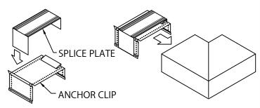
STEP 2 - MITER SPLICE PLATES & ANCHOR CLIPS REMOVE RELEASE PAPER FROM SPLICE PLATE SEALANT STRIPS. POSITION THE SPLICE PLATE IN THE CENTER OF THE ANCHOR CLIP. INSTALL THE SPLICE PLATE AND ANCHOR CLIP ASSEMBLIES HALFWAY INTO EACH END OF THE CORNER MITER AS SHOWN.
