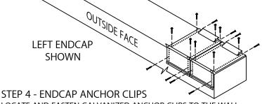
LOCATE AND FASTEN GALVANIZED ANCHOR CLIPS TO THE WALL WITH PROVIDED FASTENERS FOR SUBSTRATE, AS SHOWN IN DETAIL A. FOR FASTENER DETAIL SEE PAGE 4.
