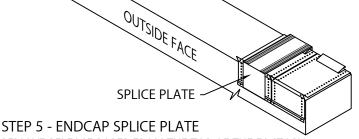
REMOVE RELEASE PAPER FROM THE TOP OF THE FACTORY APPLIED SEALANT STRIPS. PLACE THE SPLICE PLATE ONTO THE SECOND ANCHOR CLIP AS SHOWN.
