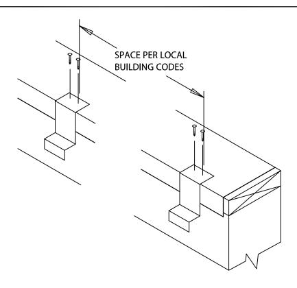
LOCATE AND FASTEN LIGHTNING ROD BRACKETS TO INSIDE FACE OF WALL PER LOCAL BUILDING CODES WITH APPROPRIATE FASTENERS FOR SUBSTRATE.
