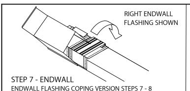
HOOK OUTSIDE FACE OF ENDWALL OVER THE ANCHOR CLIPS AND ROTATE INTO PLACE. ENGAGE REAR LEG ONTO ANCHOR CLIPS BY PRESSING DOWNWARD UNTIL SNAP LOCK OCCURS.
